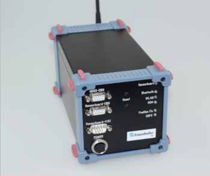
Figure 1: Development platform for seamless location by GNSS, WiFi and inertial sensors
