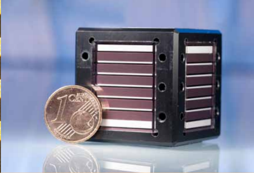
Figure 2: The solar-operated radio dice can be activated via the wake-up receiver and signals the "diced" number
