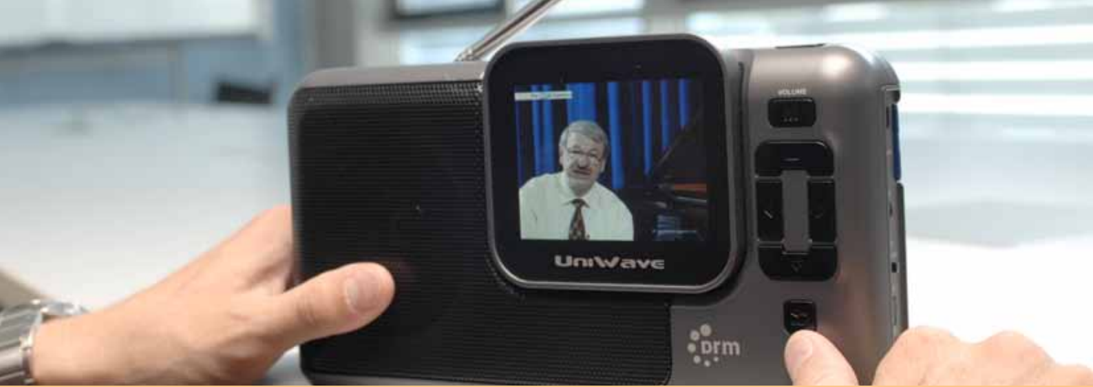
Figure 1: Diveemo-based video program on a UniWave DRM receiver
