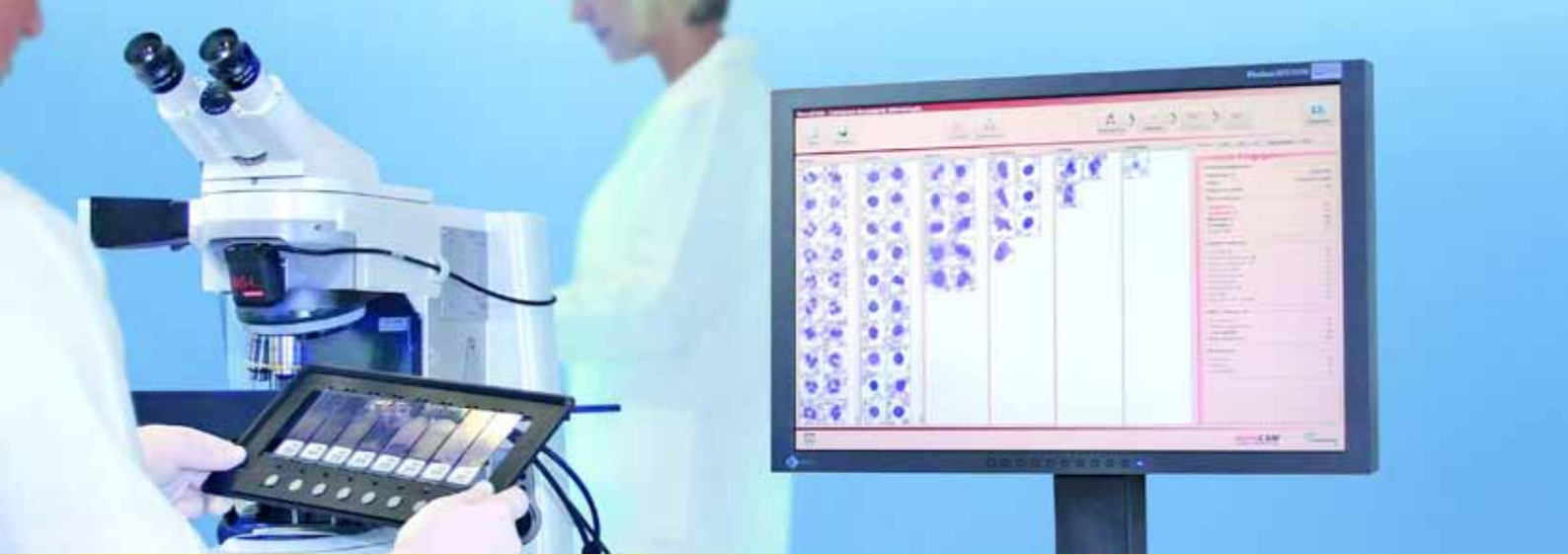
Figure 1: HemaCAM consists of a fully automated microscope with a connected camera, computer and graphical user interface and allows for automatically analyzing blood smears and supports the classification of the leukocytes
