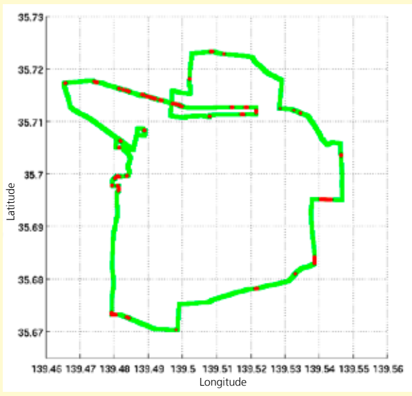
Figure: Measurements of the satellite availability along the 25 km long test route through various environments (forest, suburb and city)
